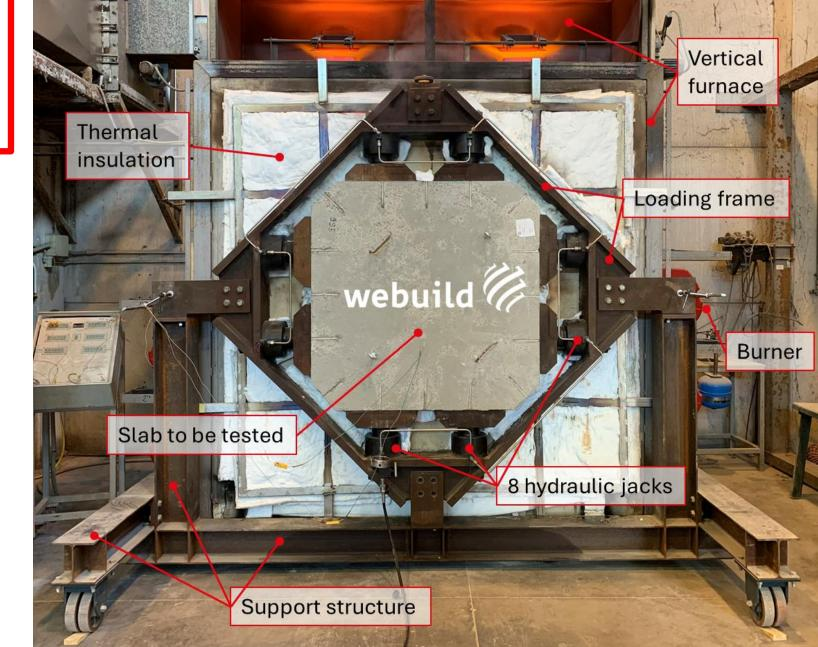
One test has been performed on a reference specimen made of SFRC with no PP fibers and another test was performed on plain reinforced concrete (without any fibre). The applied fire curve is the well-known RWS120 curve, as prescribed by the Italian railway infrastructure management (RFI) design specifications with T<sub>max</sub> of 1350°C.
