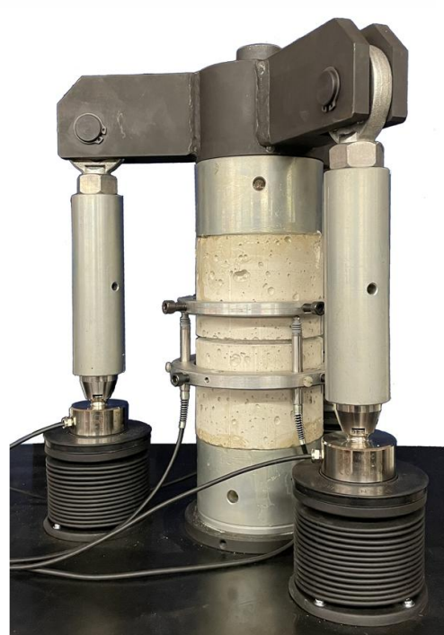
the cross-head is bolted the struts are engaged to the load cells
