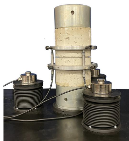
the LVDT ring supports are mounted
