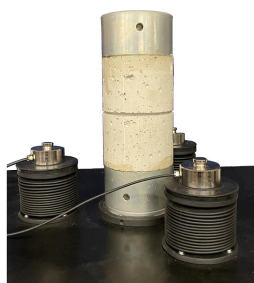
the glued steel block is screwed to the baseplate
